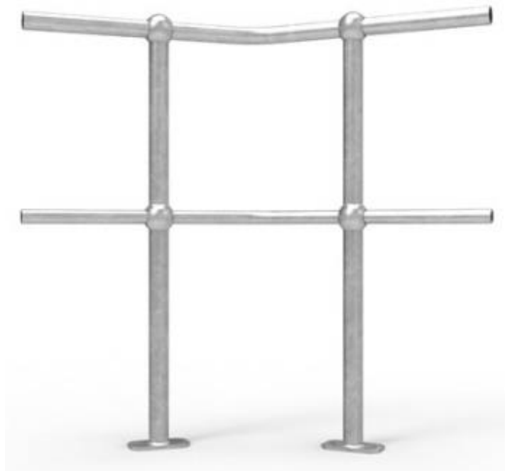
Figure 70. The equivalent Mono-Wills industrial balustrade today, not much has changed. The proposed ramp uses this balustrade along the edge of the top slab as a fall barrier, and an accessible compliant version (to AS1428 with an additional handrail and kerb rail) along the edges of the exterior ramp and landings.
